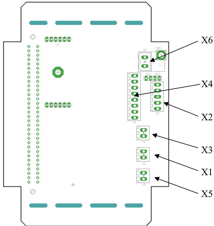
**Fig. 12 Electrical connectors / Rear view**
