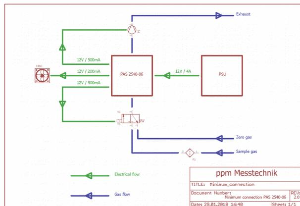
**Fig. 4 minimum connection, direct controlled accessory**
